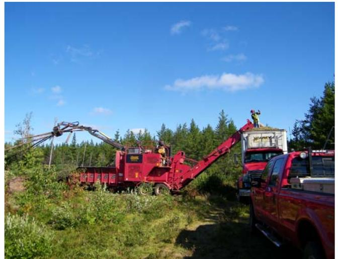
*Biomass is loaded into the chipper.*
