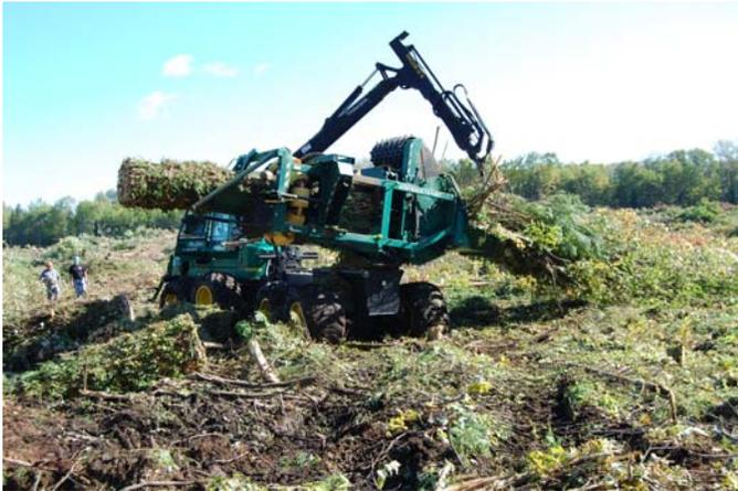
*The slash-bundler, manufactured by John Deere, is widely used in Scandinavia.*
